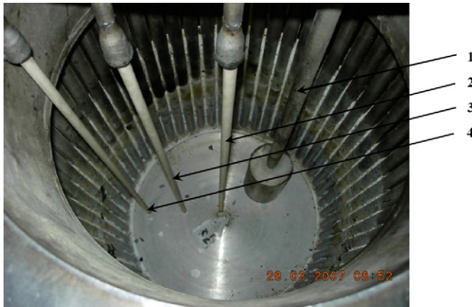
1 Mechanical plug 3 Thermowell at R = 90 mm 2 Thermowell at R = 0 mm 4 Thermowell at R = 180 mm
