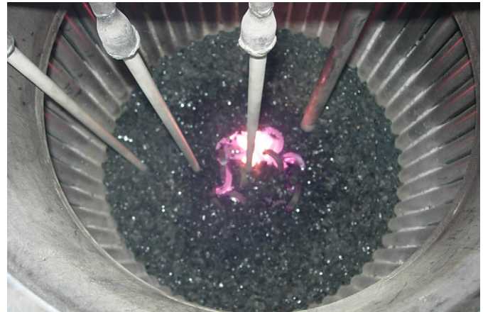
Fig. 3. Melter inside view during melter start-up.
